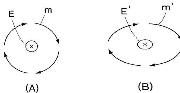
**Figure 2.** Sectional view showing the photocurrent and the photomagnetic with the polarization effect.
